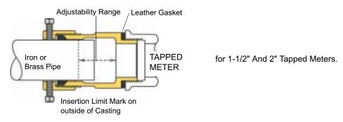
Each Coupling for a tapped meter provides adjustment of about 1". To assure space for retraction from the meter, each Coupling for tapped meters has a line on the casting to show the limit to which iron, brass or copper pipe can be inserted.
