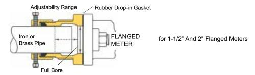
As shown in the drawing, each Lok-Pak Coupling for a flanged meter has a lateral adjustment of 2".
